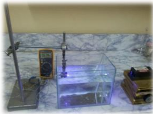
Figure 5. The setup for measuring the energy/second of photon in water.
